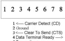
4 Data Terminal Ready 5 Transmit ---> 6 Ready To Send ----> 7 3,3Vdc 8 <---- Receive
