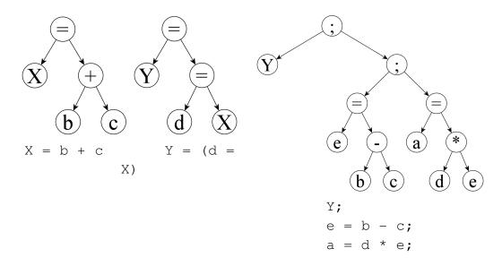
Figure 4.6: Produced program fragments and the resulting modified main program tree after the second extraction by incremental method
