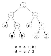
Figure 2.1: Visualisation of possible parse tree part of an input IR together with high level source code
