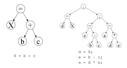
Figure 4.5: Produced program fragment and the resulting modified program tree after the first extraction by incremental method
