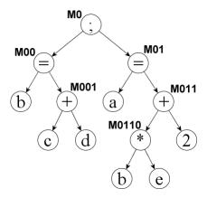
Figure 5.5: Naming of interior nodes for sample program under incremental model
