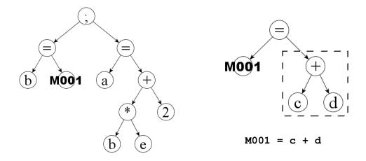
Figure 5.6: Modified parse tree and detached program segment for sample program under incremental model
