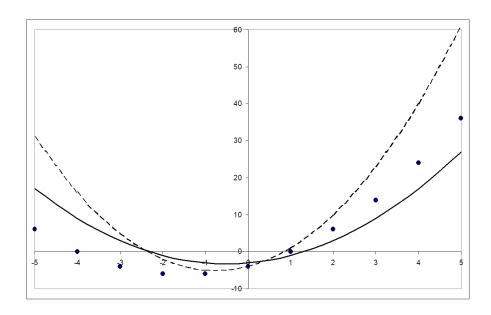
Figure 3.6: Plot of empirically obtained data set [points] together with two candidate solutions (A=1, B=1, C=-3) [dashed], and (A=2, B=3, C=-4) [solid]
