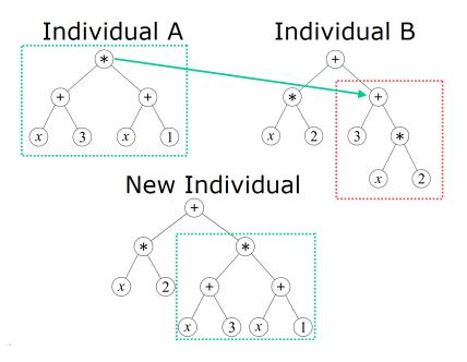
Figure 3.10: Subtree crossover in GP. The indicated subtree in Individual B is removed and replaced with the root node of Individual A to produce the New Individual
